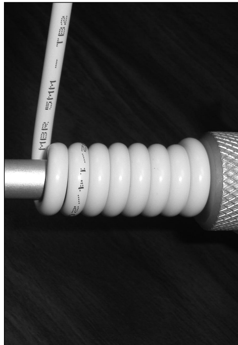
Figure 1 Bend-Insensitive Rugged Drop Cable Wound Around a Mandrel with Radius 5 mm (0.2 in)
